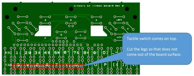
The cut is complete, remove the HT82K629A. Do not solder at this stage. Insert the tactile switches on the Front of PCB (Main Lower).
