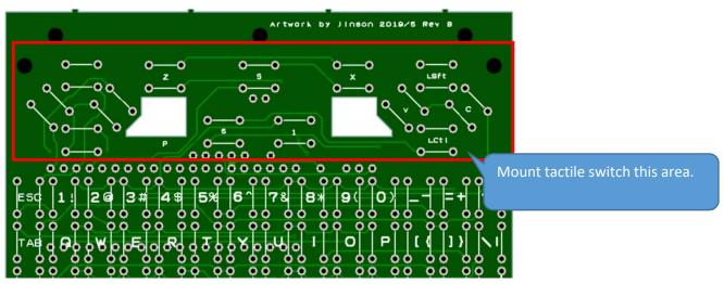
Combine PCB (Main Upper) and PCB (Main Lower) using 2.6mm x 6mm screw and nuts.
