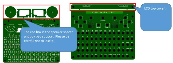
Mount the parts on the back of PCB (Main Upper).
