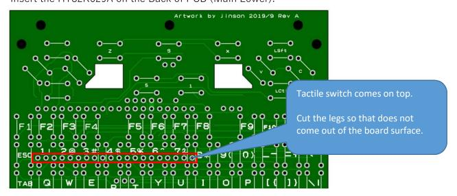
Insert the tactile switches on the Front of PCB (Main Lower).
