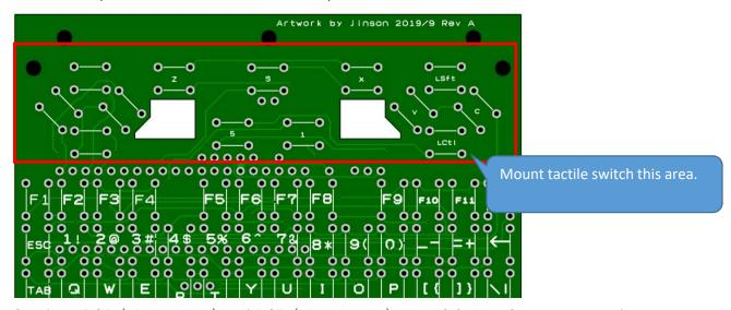
Combine PCB (Main Upper) and PCB (Main Lower) using 2.6mm x 6mm screw and nuts.
