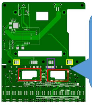
Mount the speaker spacer, which has been separated in advance, with adhesive tape to the speaker hole position. If the legs of the tactile switch comes out of the Speaker spacer board surface, cut it.
