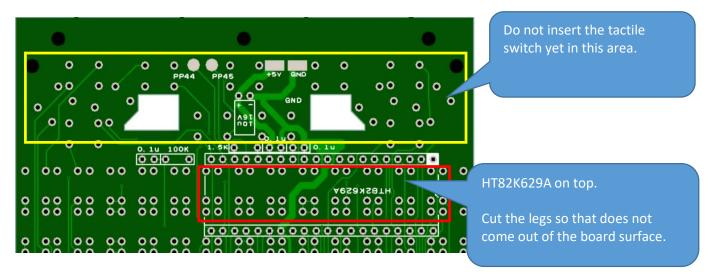
Put the front panel board and check the tactile switch shift. Solder the tactile switch if its OK.
